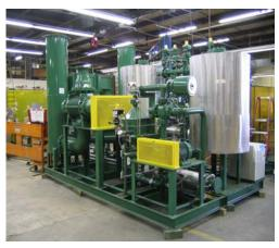
To the left is NASA's recirculating air dryer system designed for operation in a wind tun-
