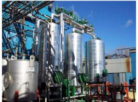
To the left is a dryer designed for a solvent recovery company drying 10,000 gallons a day of mixed solvents.
